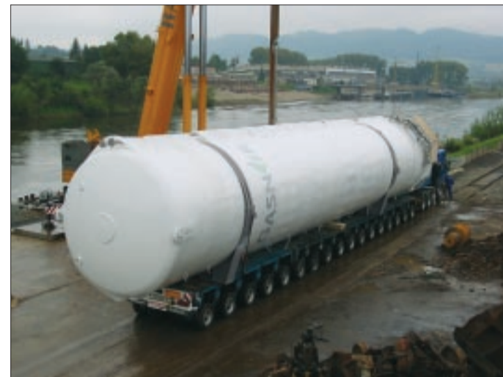
An LNG storage tank on transshipment into a ship in the Děčín port.
