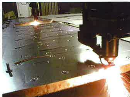
Figure 2. Laser metal fabrication shops can now enjoy the benefits of “Lights Out” operation with a reliable continuous flow of nitrogen assist gas.
